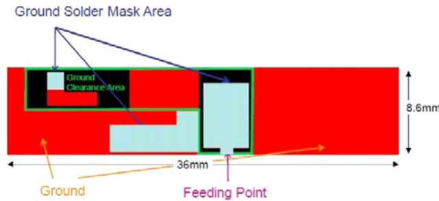
Figure 14: PCB Land Pattern of Space Saving Configuration for 1000146
