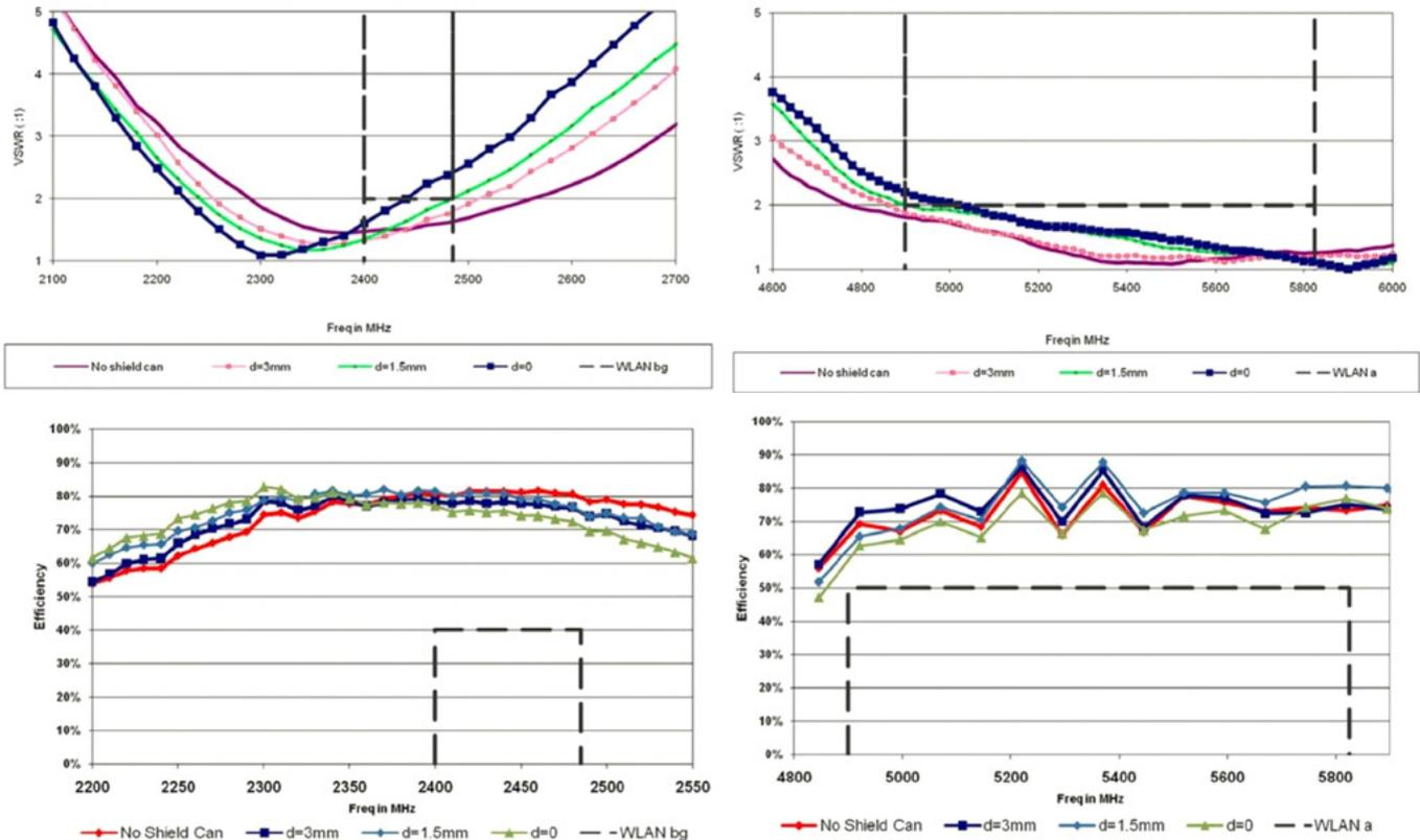
Figure 13: Shield can effect on VSWR & Efficiency of 1000146 antenna based on the distance
