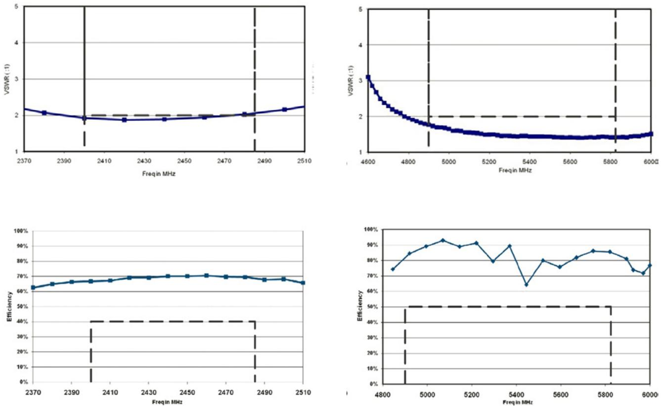
Figure 15: Space saving configuration effect on VSWR & Efficiency for 1000146
