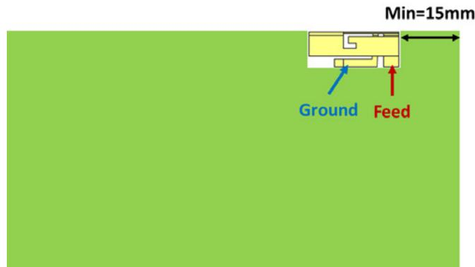
Figure 7: optimal single antenna placement for 1000146
