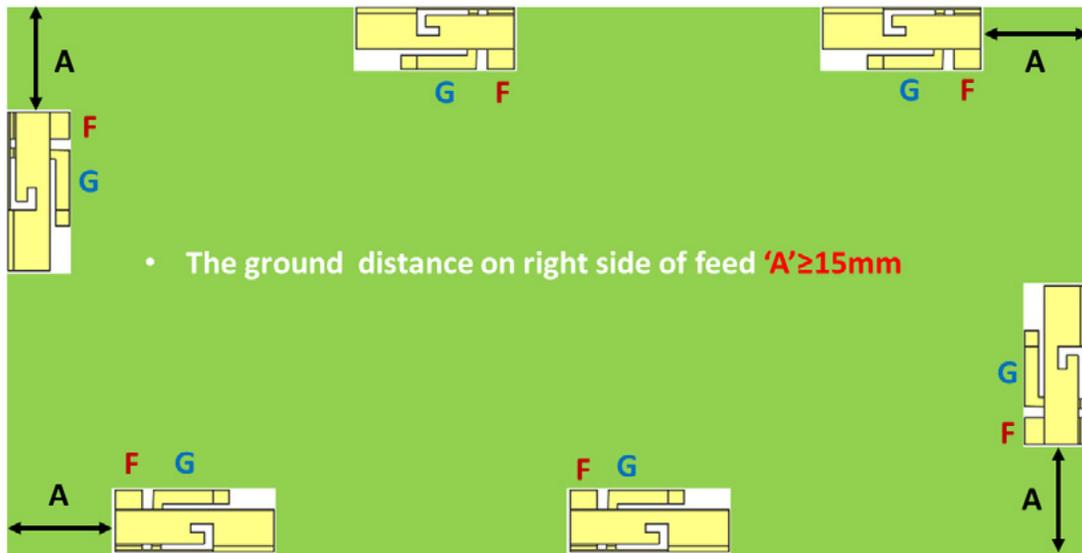
Figure 8: optimal antennas placement for 1000146 on a large PCB
