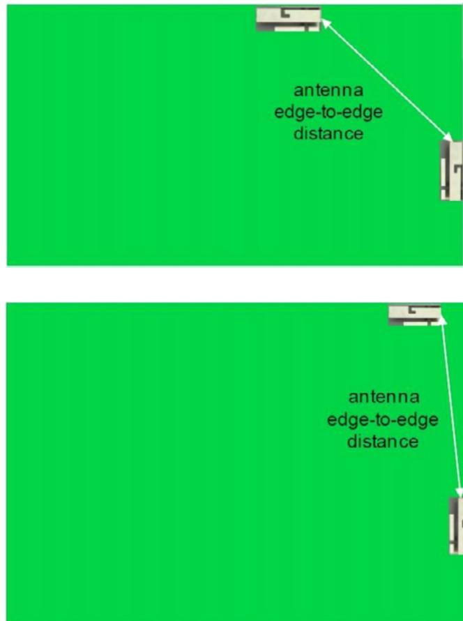
Figure 16: Recommended Layout for MIMO Applications
