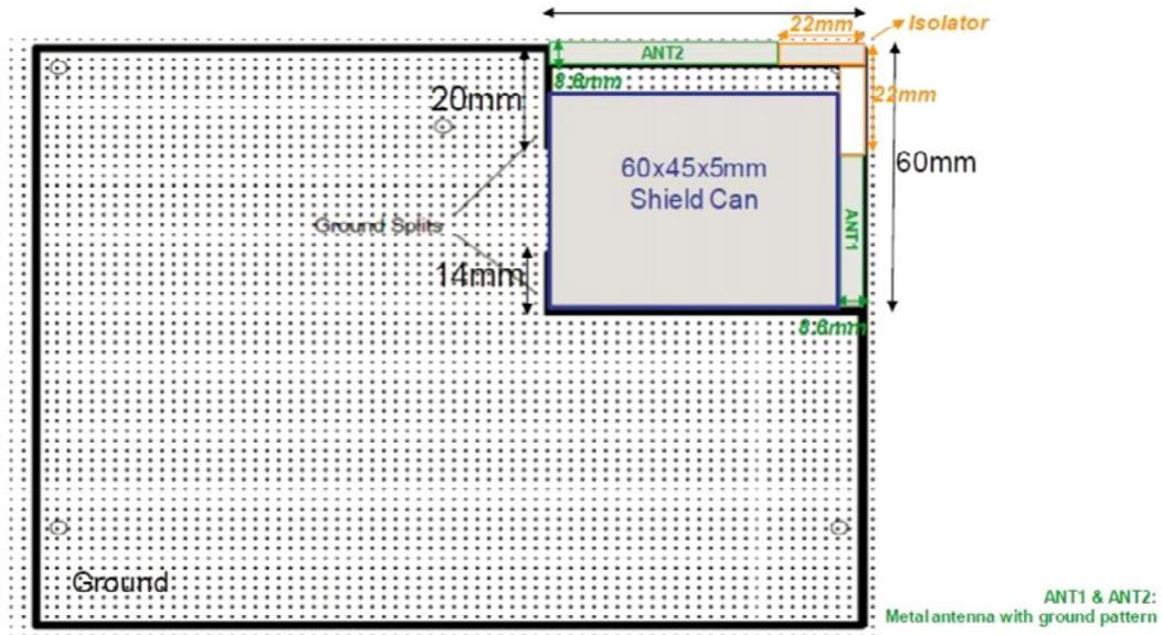
Figure 19: A Typical MIMO Configuration Example
