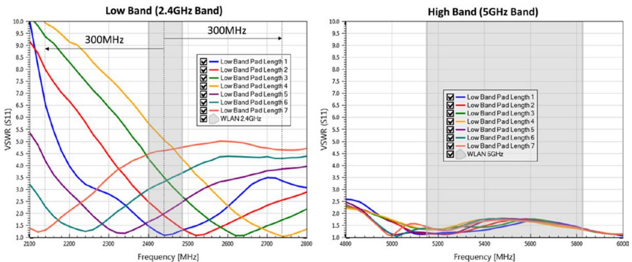
Figure 10: 1000146 Low Band Pad Configurations
