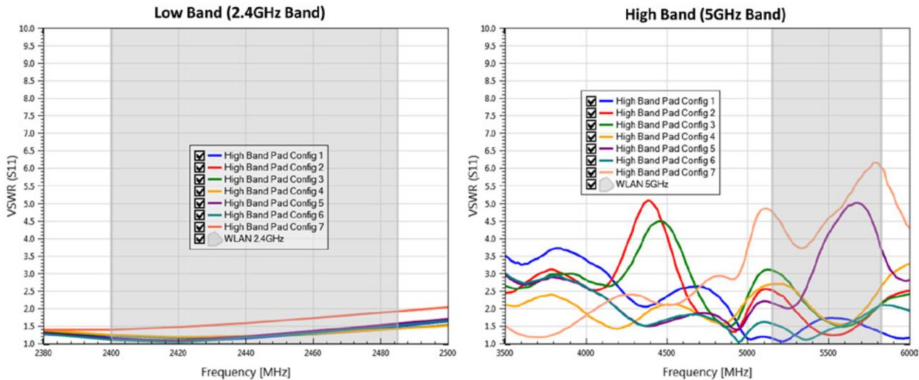
Figure 11: 1000146 High Band Tuning Pad Configurations
