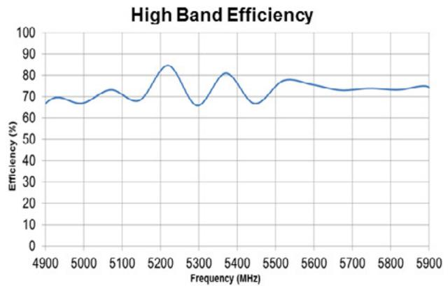
Figure 6: 1000146 Antenna Typical VSWR & Efficiency Plots on 120 x 180mm PCB
