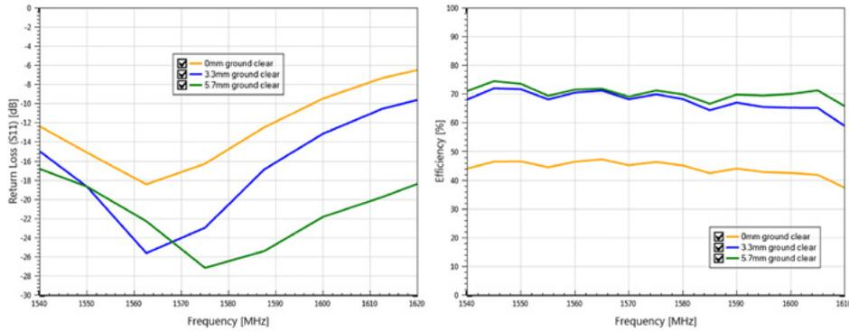
Figure 8: Ground clearance changes for 1001011
