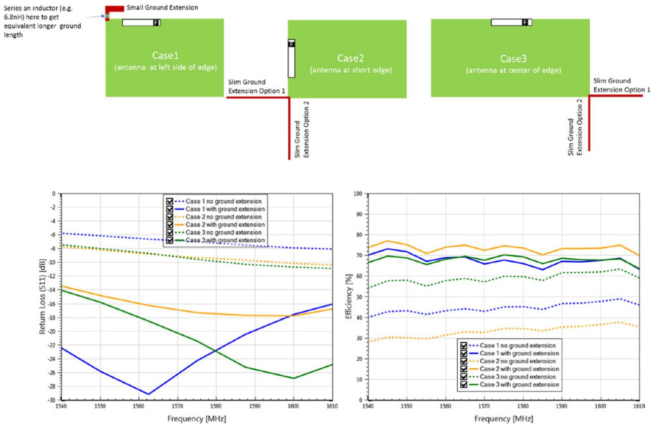
Figure 10: 1001011 antenna performance improvements with ground extensions
