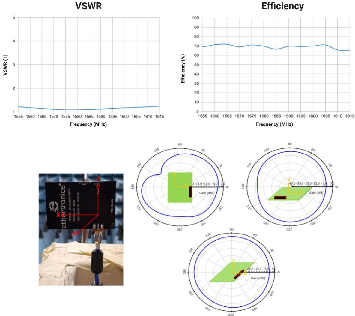
Figure 4: Typical Performance for 1001011\_Off-Ground
