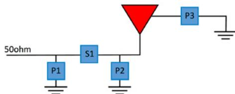
Figure 2: Antenna Layout for 1001011 Off-Ground
