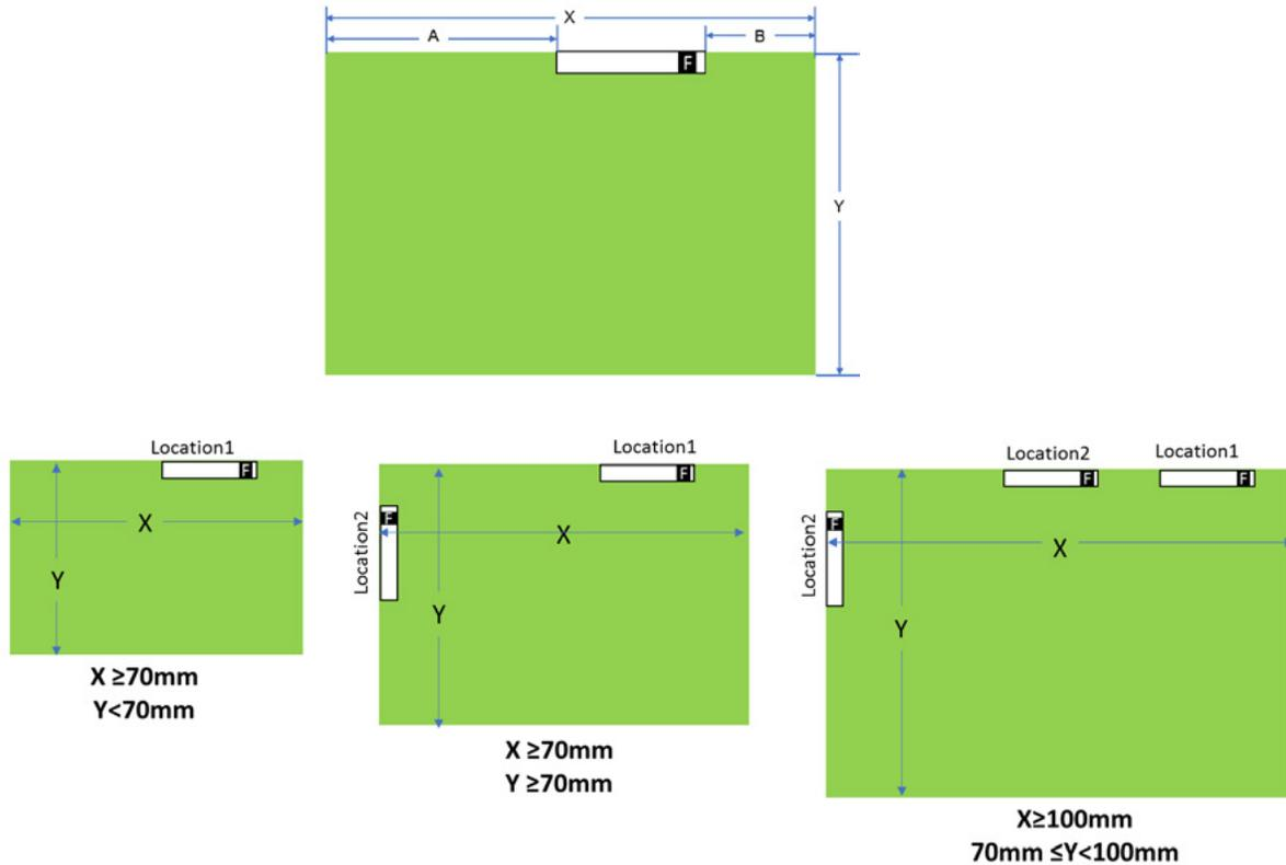
Figure 6: Optimal placement of the 1001011 on a PCB
