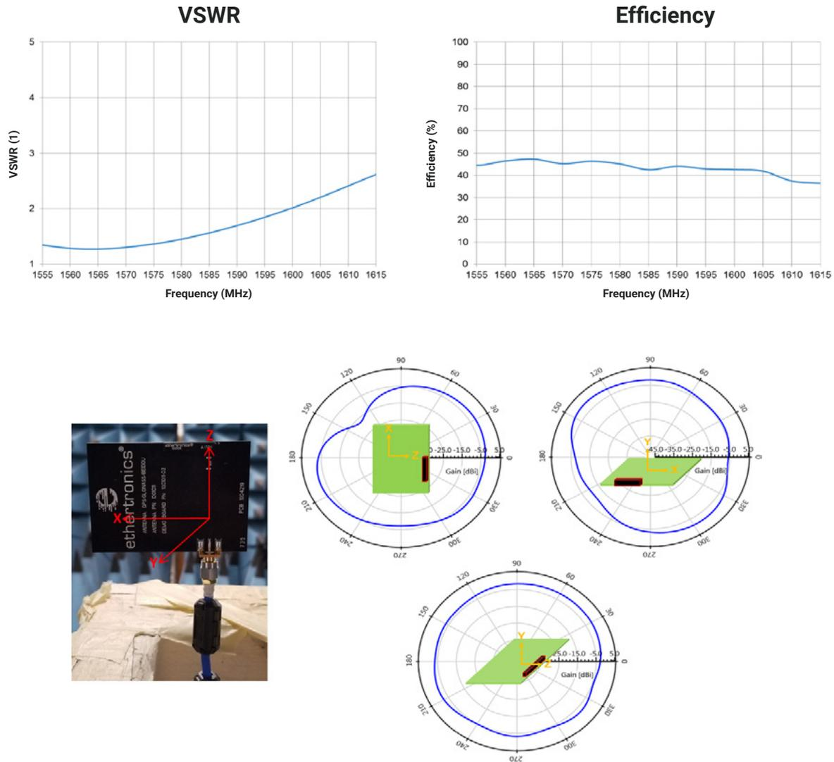
**Figure 5: Typical Performance for 1001011\_On-Ground**
