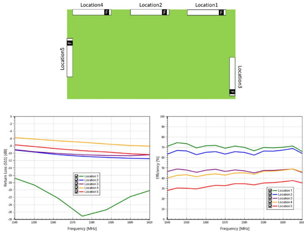
Figure 9: 1001011 antenna on different board locations
