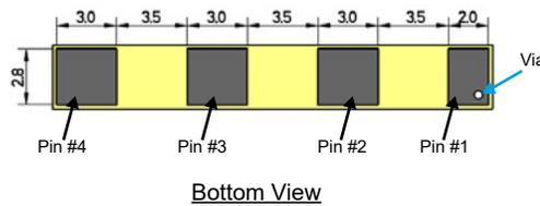
Figure 1 : Antenna Dimensions and Pad Layout for 1001011
