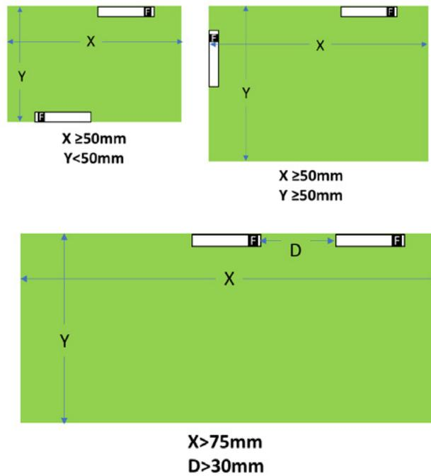
Figure 11: 1001013 Typical MIMO Configurations
