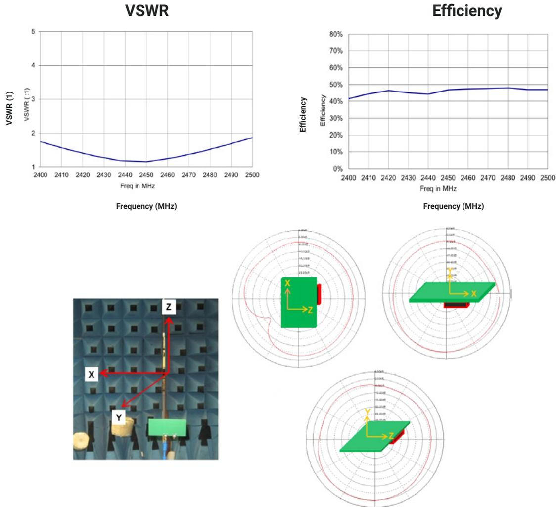
**Figure 5: Typical Performance for 1001013-1 (On-Ground)**
