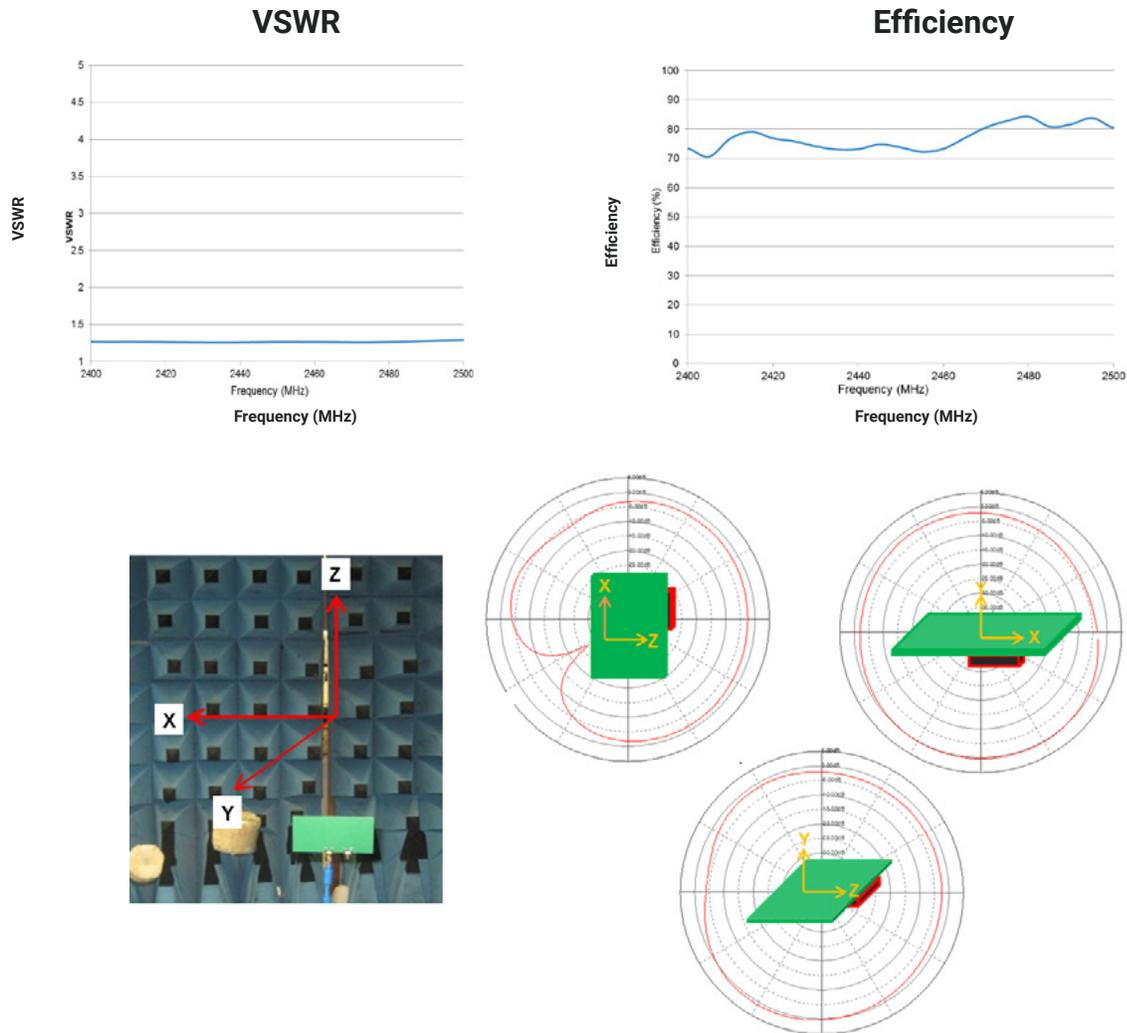
Figure 4: Typical Performance for 1001013-02 (Off-Ground)
