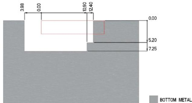
Figure 2: Antenna Layout for 1001013-02 (Off-Ground)
