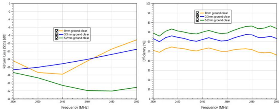
**Figure 8: Ground clearance changes for 1001013**
