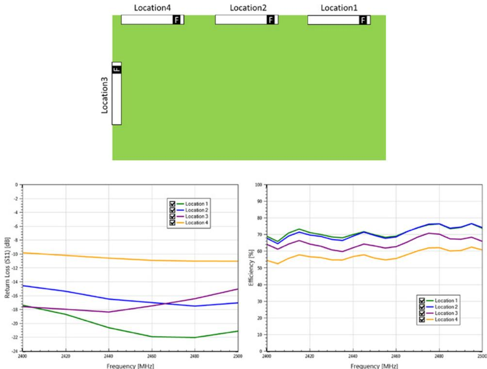
**Figure 9: 1001013 antenna on different board locations**
