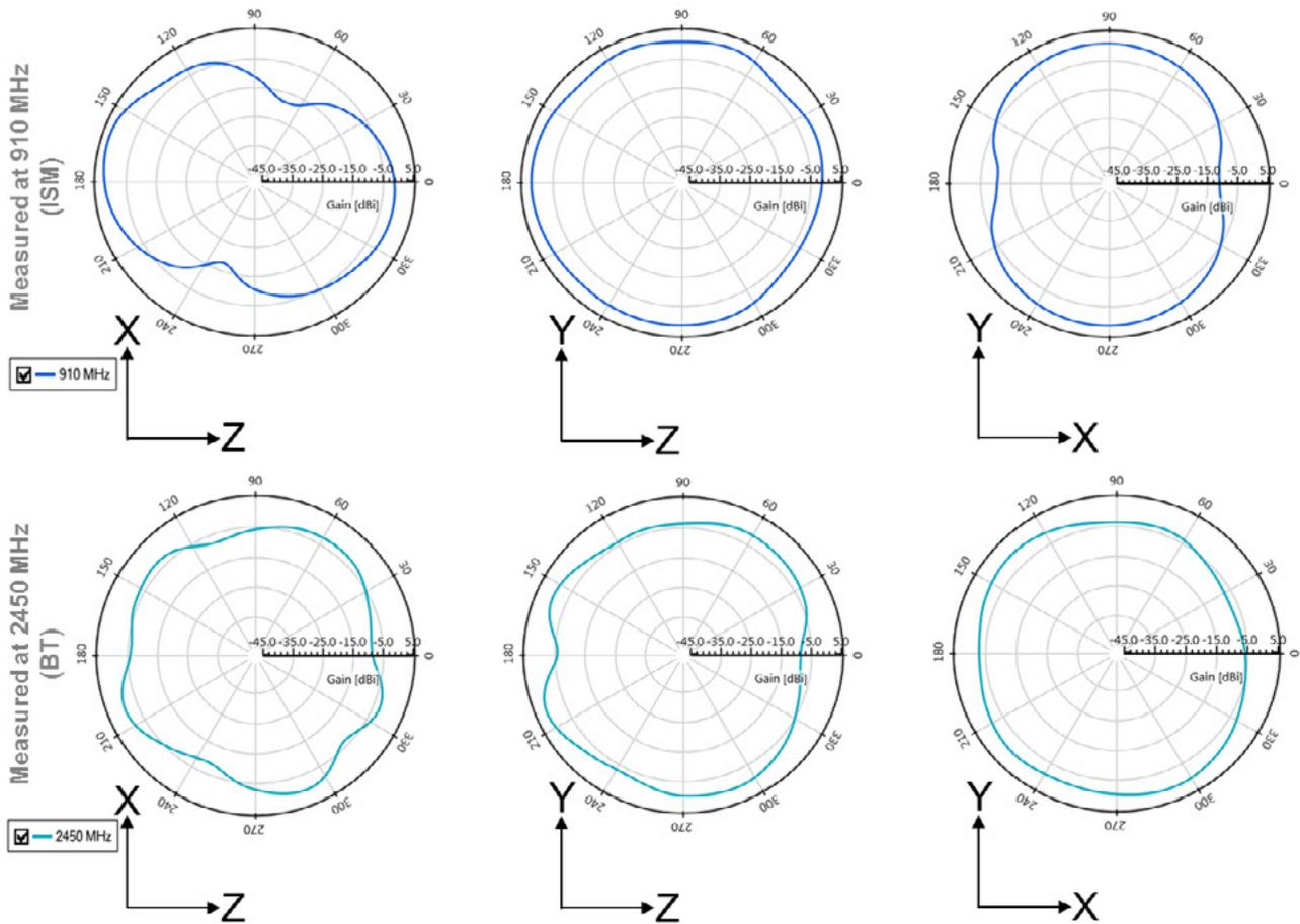
Figure 6 : 1002427 Antenna Typical Performance for ISM & BT Dual Band
