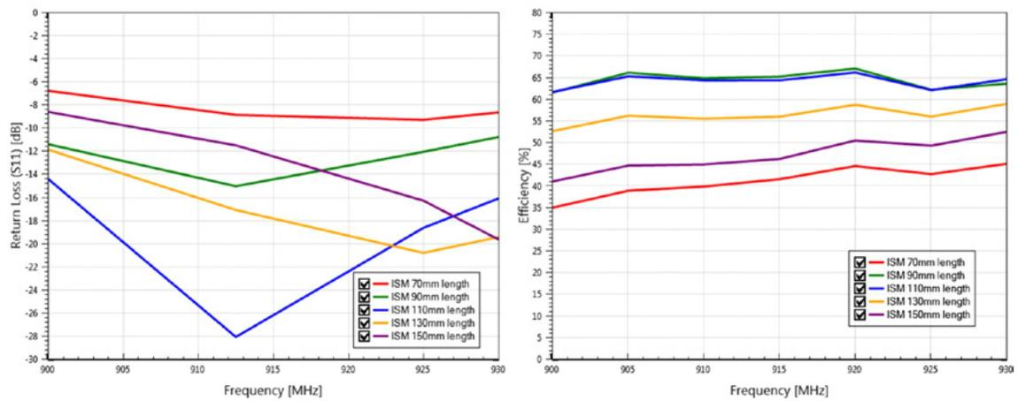
Figure 17 : 1002427 ISM ONLY performance varies with different PCB length
