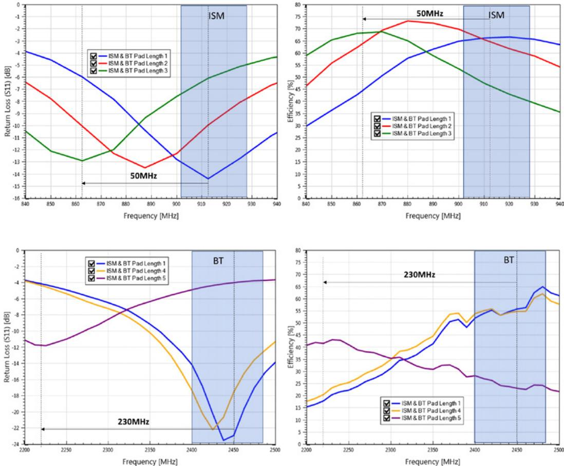
Figure 10 : 1002427 ISM & BT Dual Band Tuning Pad Configurations
