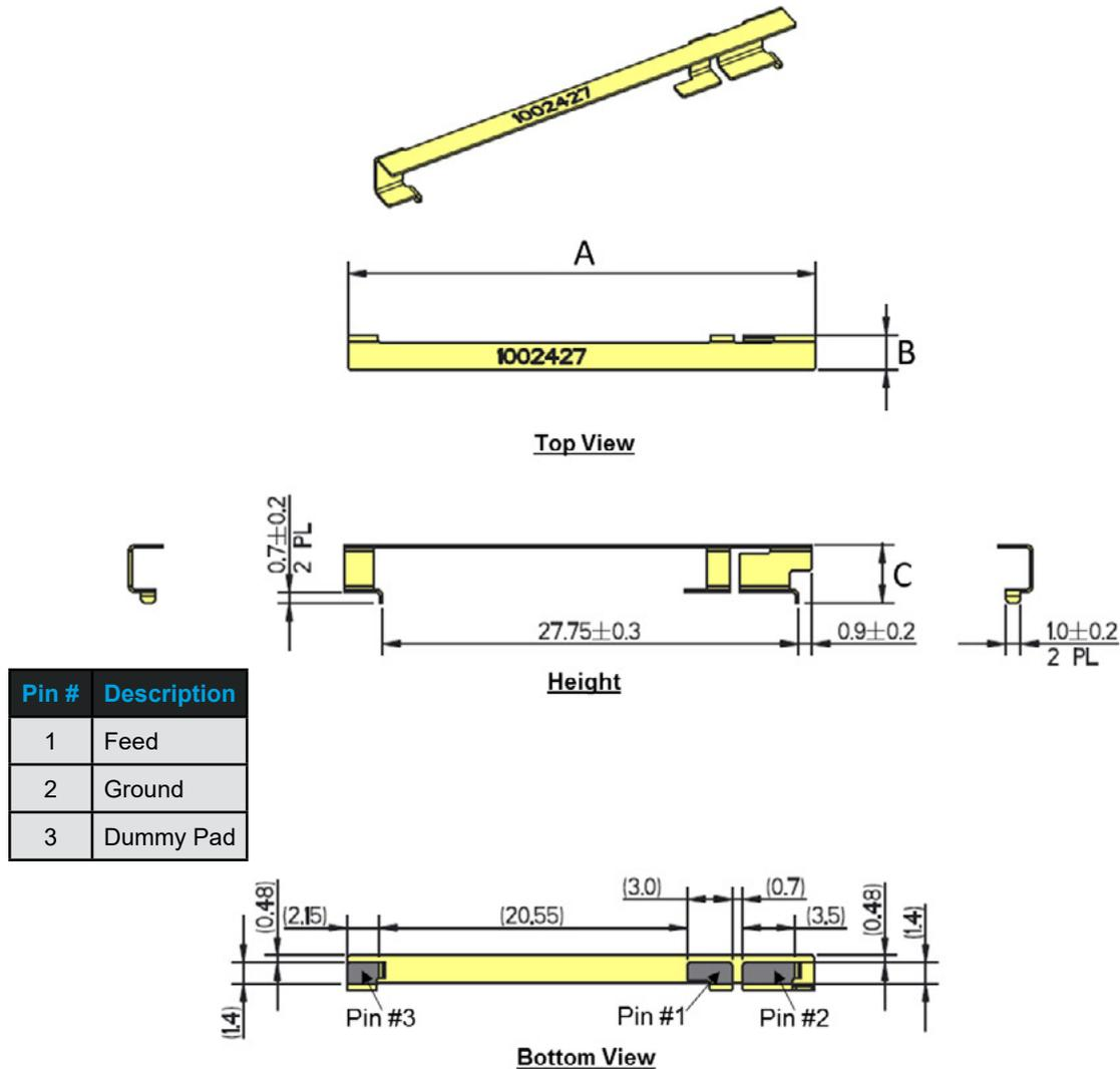
Figure 1 Antenna Dimensions for the 1002427
