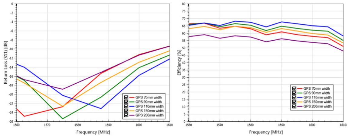
Figure 16 : 1002427 GPS ONLY performance varies with different PCB width
