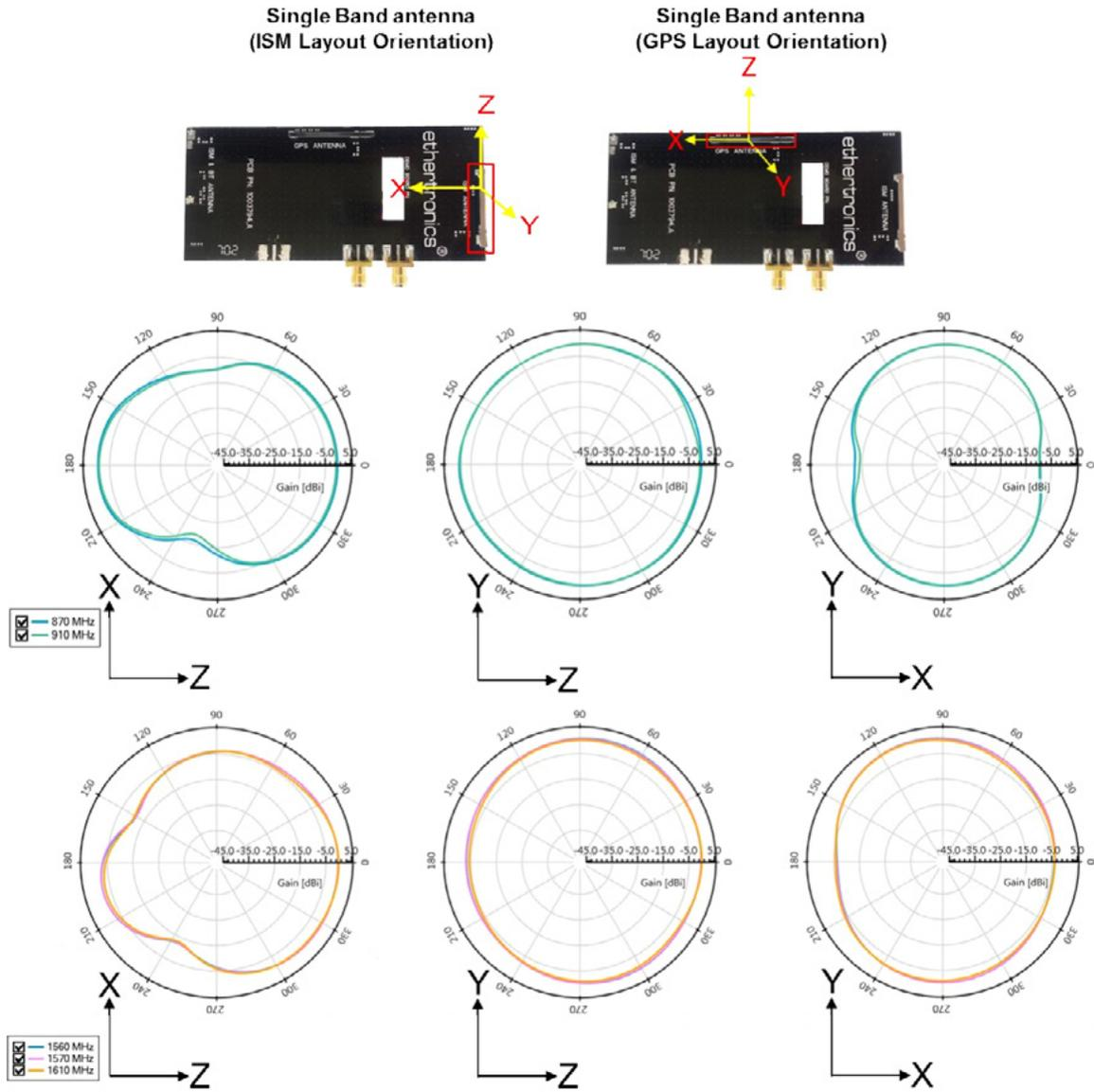
Figure 5 : 1002427 Antenna Typical Performance for GPS ONLY and ISM ONLY
