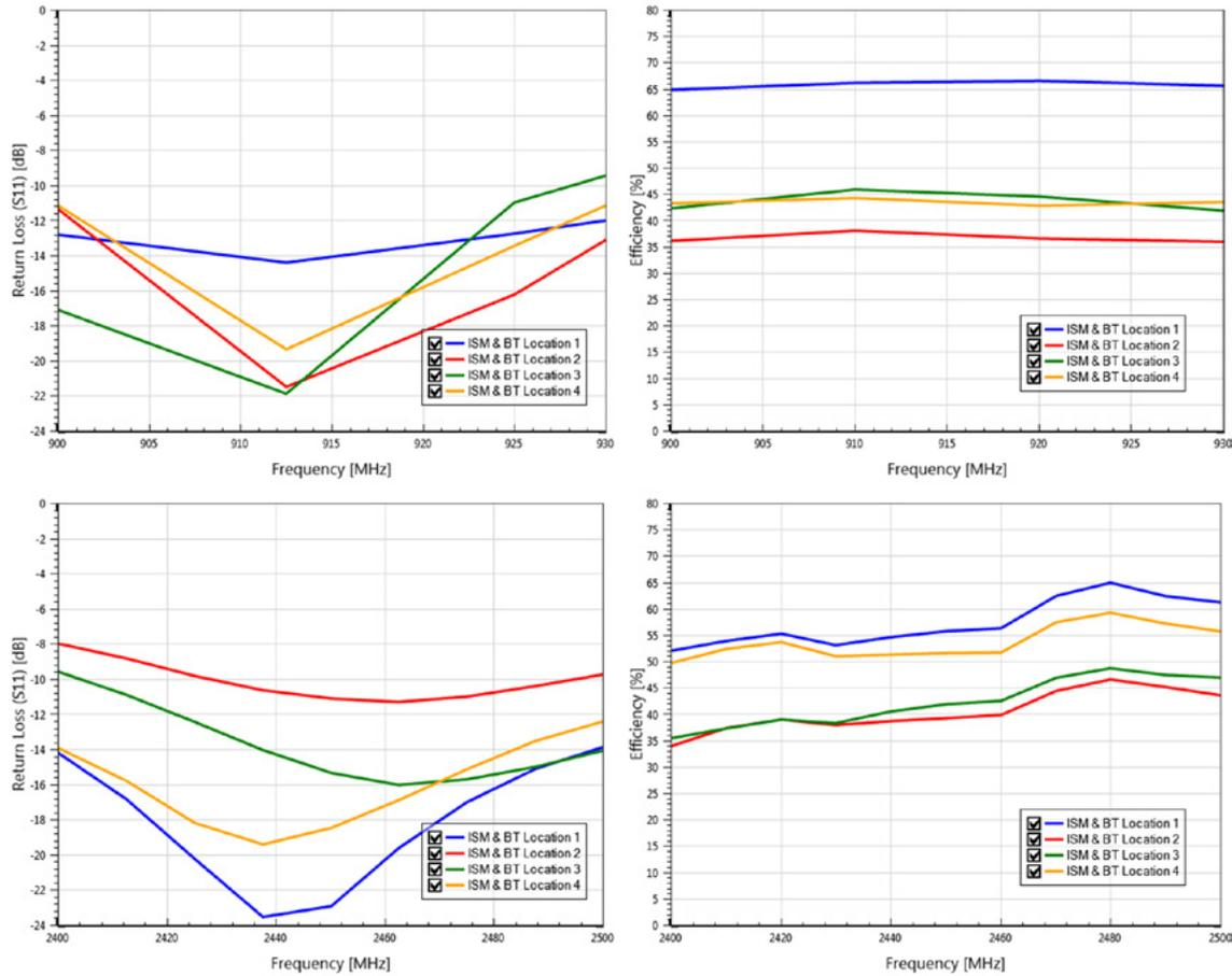
**Figure 14 : 1002427 ISM & BT Dual Band with Four Locations**
