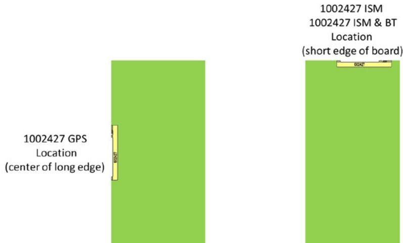
Figure 7 : 1002427 typical landing location for each antenna layout
