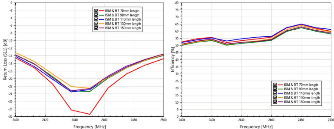
Figure 18 : 1002427 ISM & BT performance varies with different PCB length
