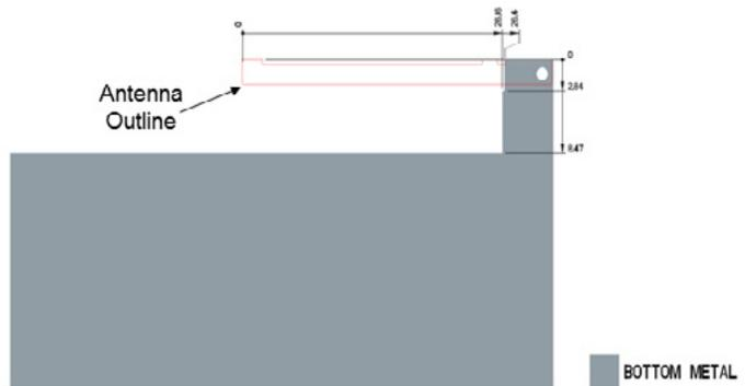
Figure 4 : 1002427 Antenna Footprints for ISM & BT Dual Band
