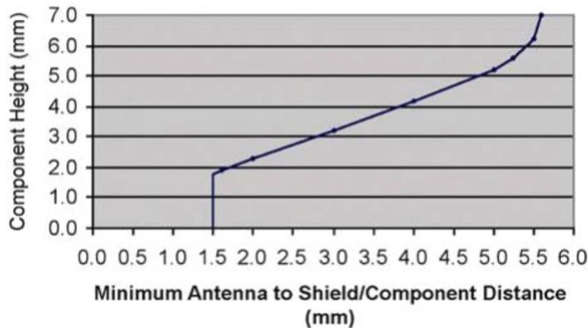
Figure 7 above shows the Minimum Antenna - Shield and/or Component Distance
