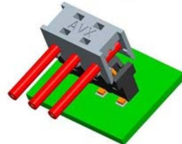
3. Push down on cap until clips latch on the connector
