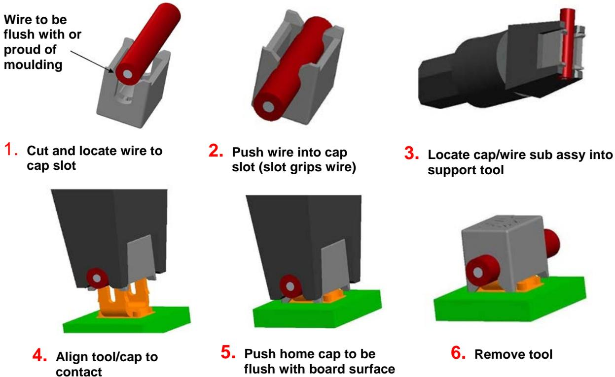
Typical insertion force is approximately 175N per wire for -400 series and 225N per wire for -500 series. This is dependent on the wire gauge, conductor strands and insulation material.
