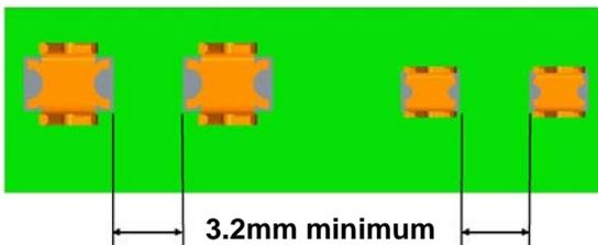
UL approval based on 3.2mm gap between pads.
