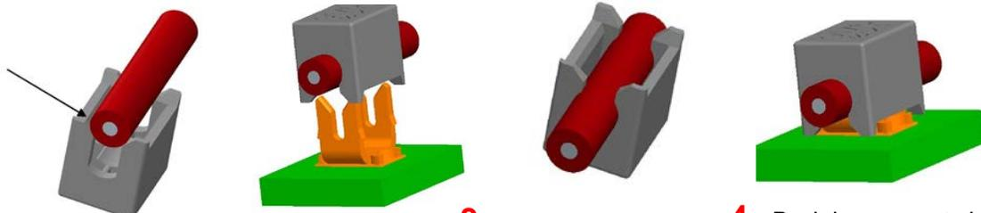
1. Cut and locate wire to cap slot
