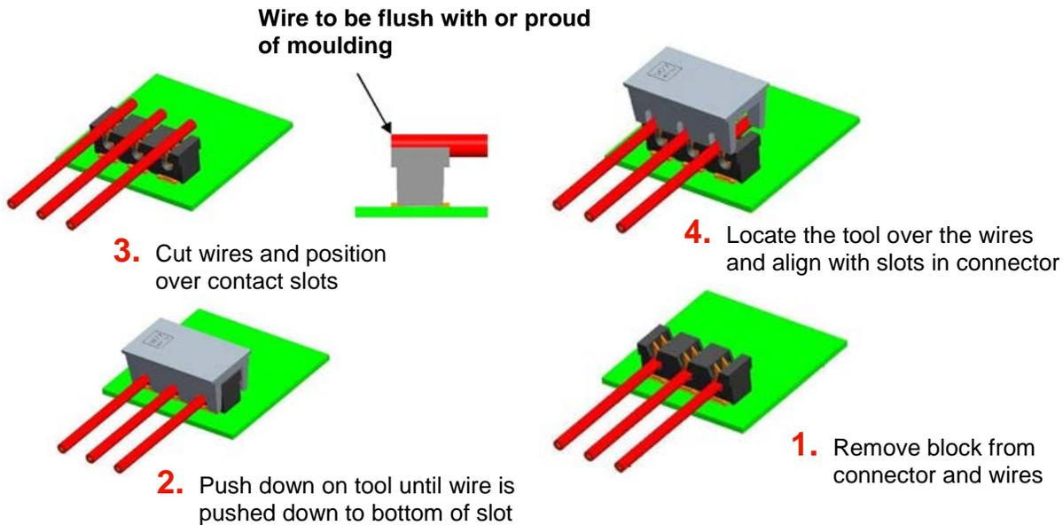
Typical insertion force is 250N to 350N per wire, this is dependent on the wire gauge, number of conductor strands and insulation material.
