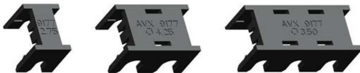
**9177 Cap:** Available in 1way, 2way and 3 way with through wire and wire stop options. Sizes 2.75mm, 3.50mm and 4.25mm wire insulation diameter for 14AWG to 20AWG wires.
