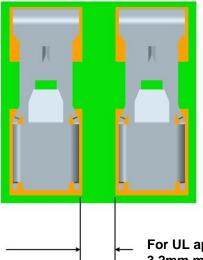
UL approval based on 3.2mm gap between pads.
