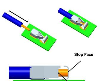
Wires are inserted through the front aperture of the contact. They should be pushed beyond the grips up to the stop face.
