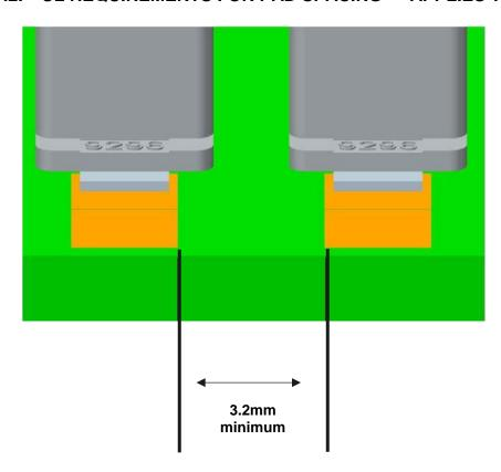
UL approval based on minimum 3.2mm spacing between pads.
