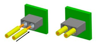
Wires are inserted through the front aperture of the connector.
