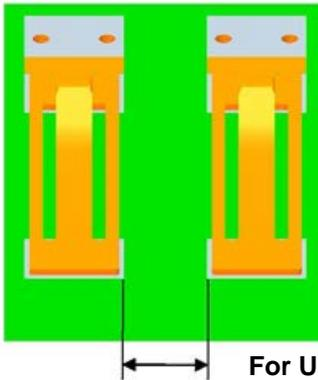
UL approval based on 3.2mm gap between pads, contact centre spacing 5.9mm.
