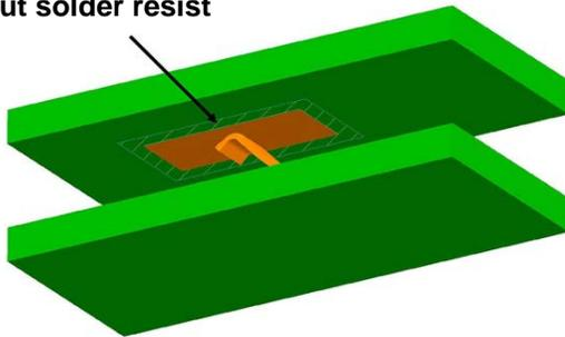
A single pad plated with gold over a nickel under-plate is recommended for good contact under all conditions. Dimensions of pad refer to sales drawing. An area around the mating pad approximately 0.5mm wide should be free of solder resist. This prevents the contact nose riding up on the resist and losing contact with the pad, see also section 4.2 on misalignment above.
