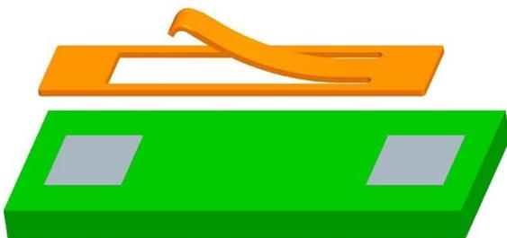
2 solder pads, refer to sales drawing for dimensions. Placing a pad between these is not recommended as it may affect contact performance. The space between the pads should be kept clear of all tacks and components. It is recommended that solder pads are tin plated.
