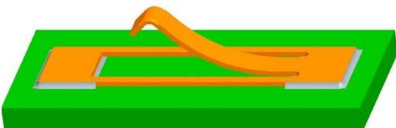
After SMT the contact should be sitting square on the pads and have small fillets all around soldered edges.
