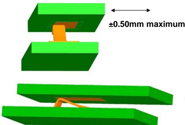
The recommended PCB mating pad layout has been designed to cope with a generous tolerance for misalignment between boards of  $\pm 0.50\text{mm}$  side to side and 1.50mm end to end. These tolerances should be regarded as a maximum and in practice we recommend that the misalignment is kept to a minimum.
