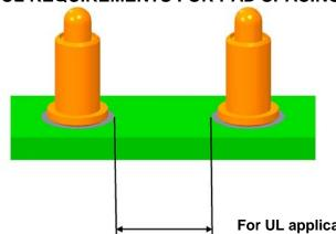
UL approval based on 3.2mm gap between pads, contact centre spacing 5.6mm.
