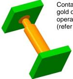
Contacts should be mated to a pad plated gold over nickel and set at the correct operating height (H) for the contact used (refer to sales drawing).
