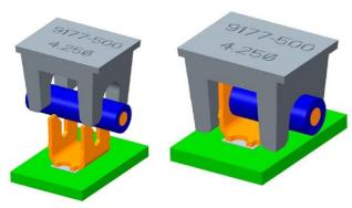
3. Place the tool over the wire insulation, there should be a small overlap at the end (2.0mm minimum). It is important to choose the correct tool to match the insulation diameter.
