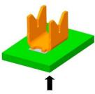
1. It is important to support the underside of the PCB during the assembly procedure.
