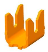
SMT mount contacts available in each of 4 wire sizes 12AWG, 14AWG, 16AWG and 18AWG, either solid conductor or most stranded conductor styles. Refer to sales drawing for correct contact part number for wire gauge used.
