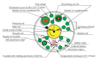
This metallized film results in the principle of selfhealing which is the major reason for the increase in gradient of voltage. Even if polymer quality improves a lot, main developments are done on metallization.
