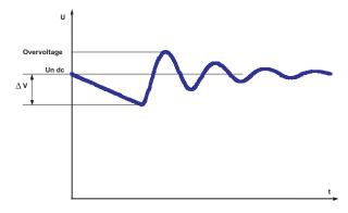
Due to the principle of carrying the power from the catenary's to the train, some contact discontinuity appears between pantograph and catenary's.
