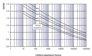
As we can see on these curves, design is done for a lifetime of 100,000 hours under the rated voltage and  $70^{\circ}$ C hot spot.
