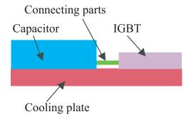
On the example above, capacitor is directly screwed onto the IGBT module, using its own terminals.
