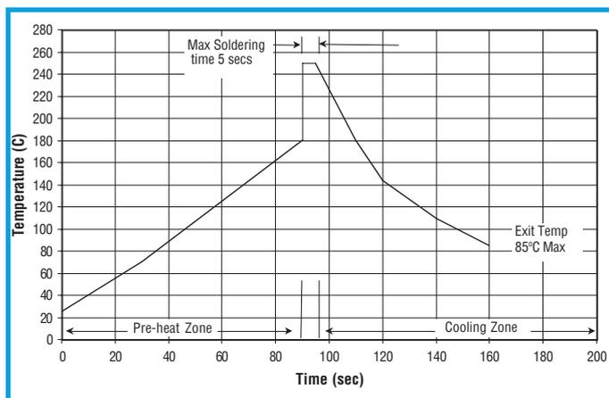
Figure 2. Typical Wave Solder Profile
