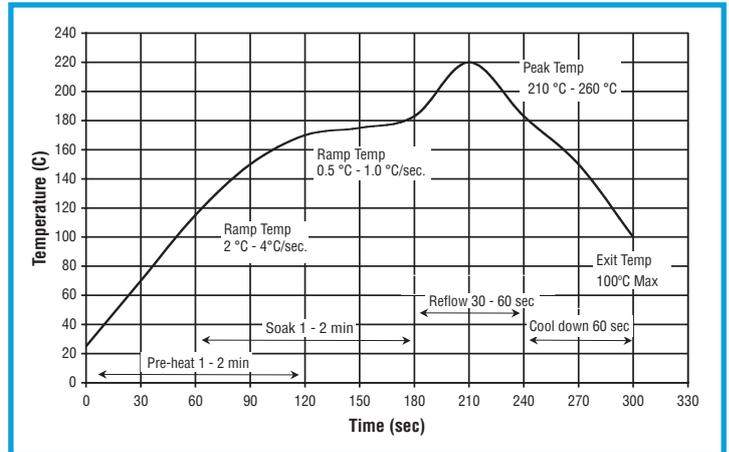
Figure 1. Typical Infrared or Convection Reflow Profile
