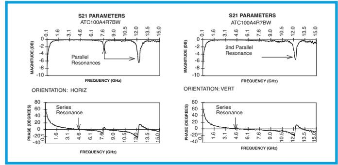
**Figure 3.** S-Parameter Plots comparing horizontal and vertical mounting orientations
