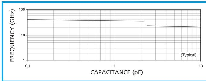
**Figure 1.** Typical first parallel resonant frequency.
