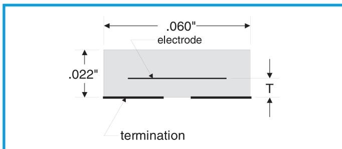
**Figure 2.** Typical longitudinal cross section.
