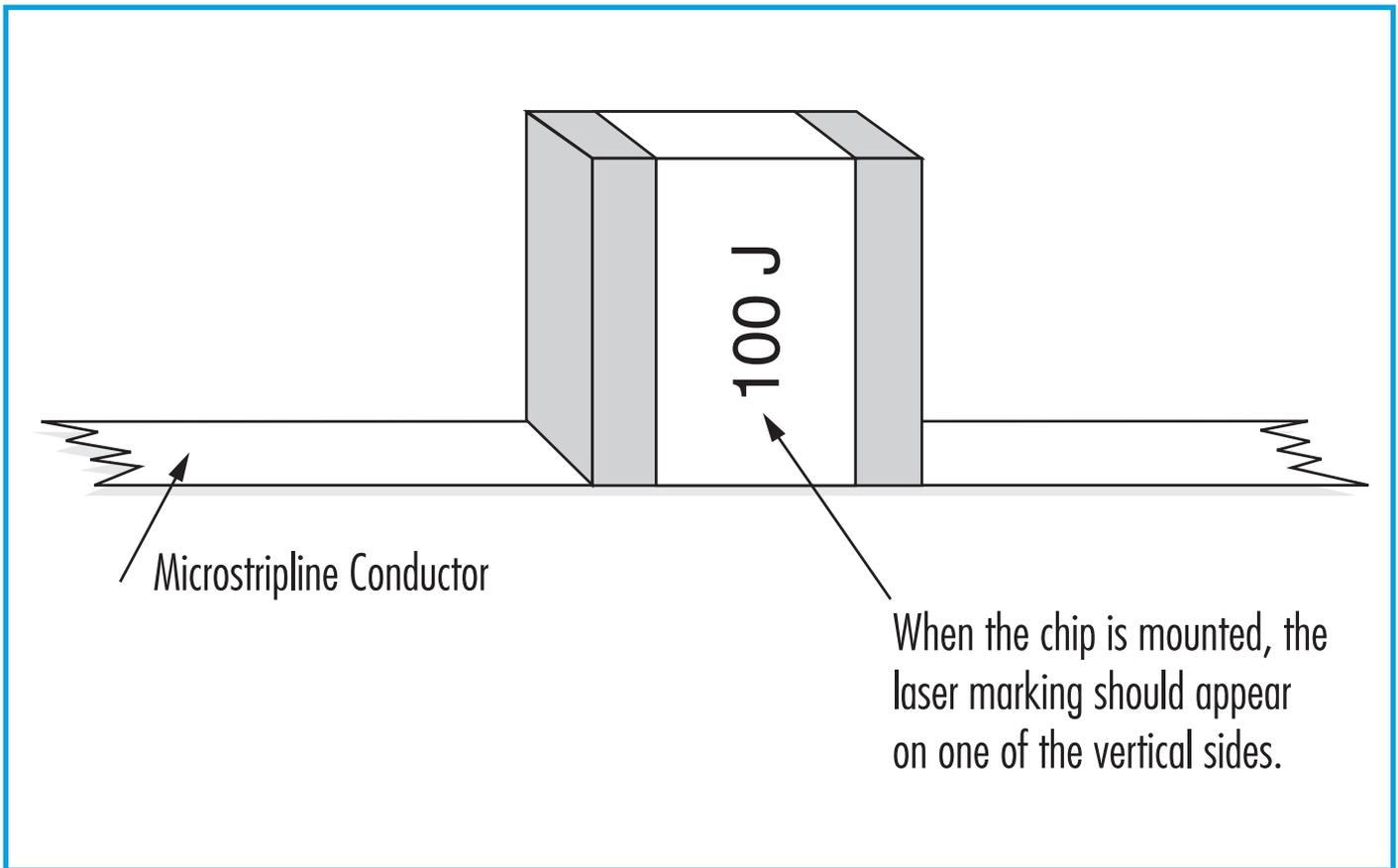
You may order a HN or HS style capacitor having narrow microstrip leads such that the capacitor plates are in the orientation shown in the illustration.
