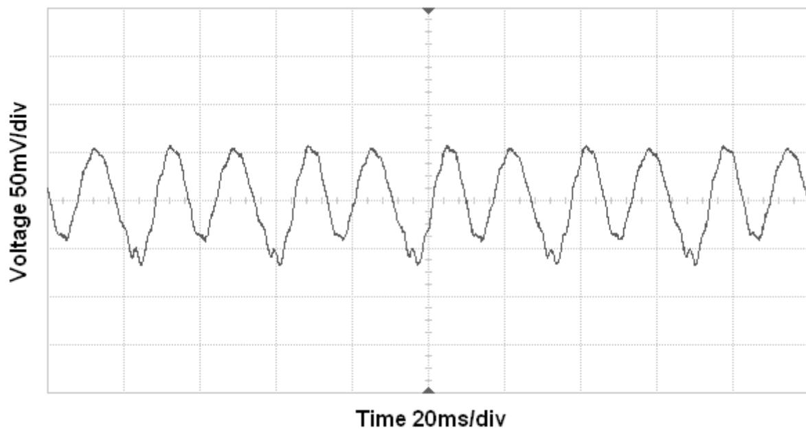
*Figure 3: AC output voltage of the PFCB-W14 piezo element when loaded by 1kΩ resistor*
