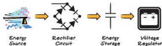
Figure 4: Principle of the energy harvesting system
