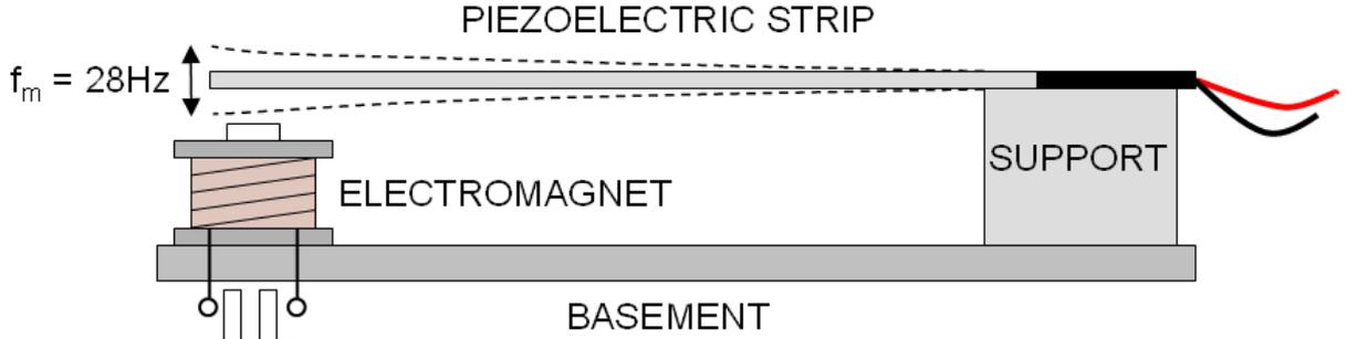
Figure 1: Experimental piezoelectric generator using PFCB-W14 element
