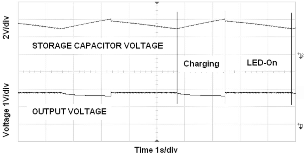
Figure 6: Output voltage and Storage capacitor voltage showing Charging phase and LED-On phase. NOTE: 0V indicators ('1', '2')
