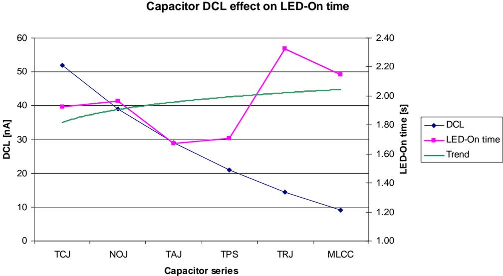
Figure 9: Storage capacitor DCL effect on LED-On time
