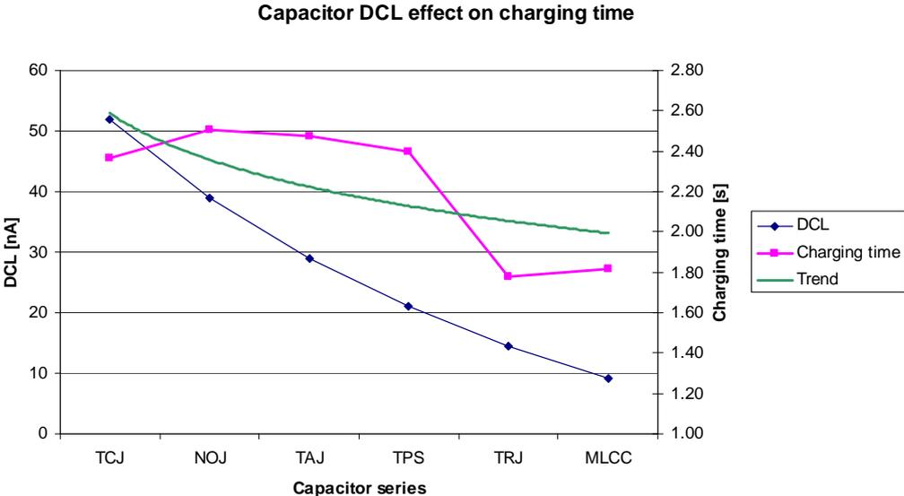
Figure 8: Storage capacitor DCL effect on charging time
