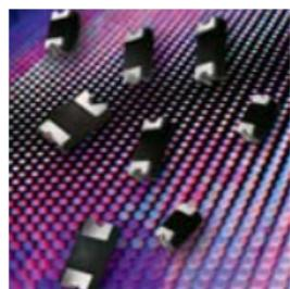
AVX Schottky rectifier diodes offer unique lead-less chip packaging technology which eliminates the lead frame wire bond to give the chip top-bottom symmetry for fewer mounting problems, better heat transfer, and current handling capability (compared to SOD devices). EIA 1206 size Schottky diodes with forward voltage as low as 0.38V and working voltage range of 20V to 100V. All AVX SD Series diodes are equivalent in footprint to JEDEC sizes.
