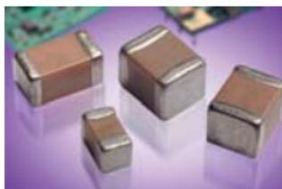
X5R dielectric is a Class II type dielectric suitable for higher capacitance applications. This dielectric offers high volumetric efficiency. Small case size X5R capacitors are well suited for decoupling and filtering applications in mobile devices and other applications with size constraints.
